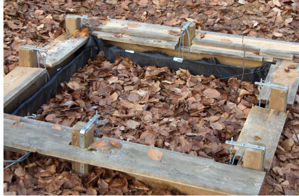
Figure 2.5: Forest floor device in the Huewelerbach with a beech layer.
