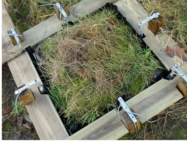
Figure 2.6: Forest floor device in Westerbork with a moss/grass layer.
